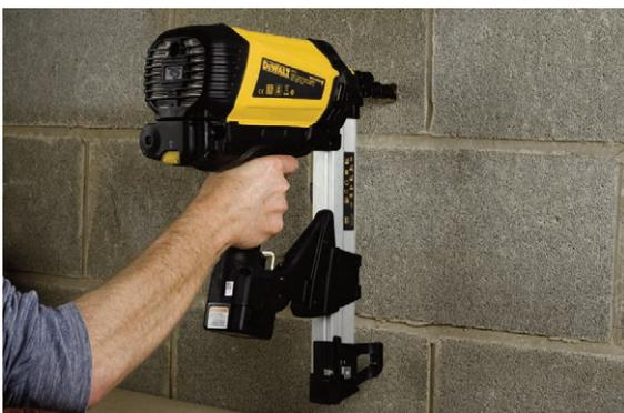
If you have larger numbers of fixings to make in one go, particularly straight onto brickwork, blockwork or concrete, then gas nailing is the way to go. In our trials, we used the *DeWalt® C5 gas nailer* with *25mm XC nails*. Once set up, the gun will fix nails straight through the pre-formed hole or even through the clip itself regardless of the density of the substrate. Using the harder XH nails even allows for fixing directly to steel work if that is the way the circuit is routed.
