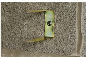
*Walldogs®* work well when fixed either directly to substrate or within PVC trunking (25mm to 50mm sizes). Simply drill the pilot hole straight through the pre-formed hole in the clip, the back of the trunking and directly into the wall behind.
