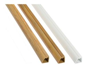
% round 22 x 22mm profile covers expansion gaps between floors and skirting. The 22 x 22mm (W x H) dimensions scale well to blend with popular skirting boards, while providing capacity for cable bending radii around corners.
