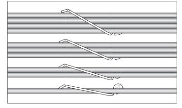
• The spring-tensioned arm drops over to secure cables
